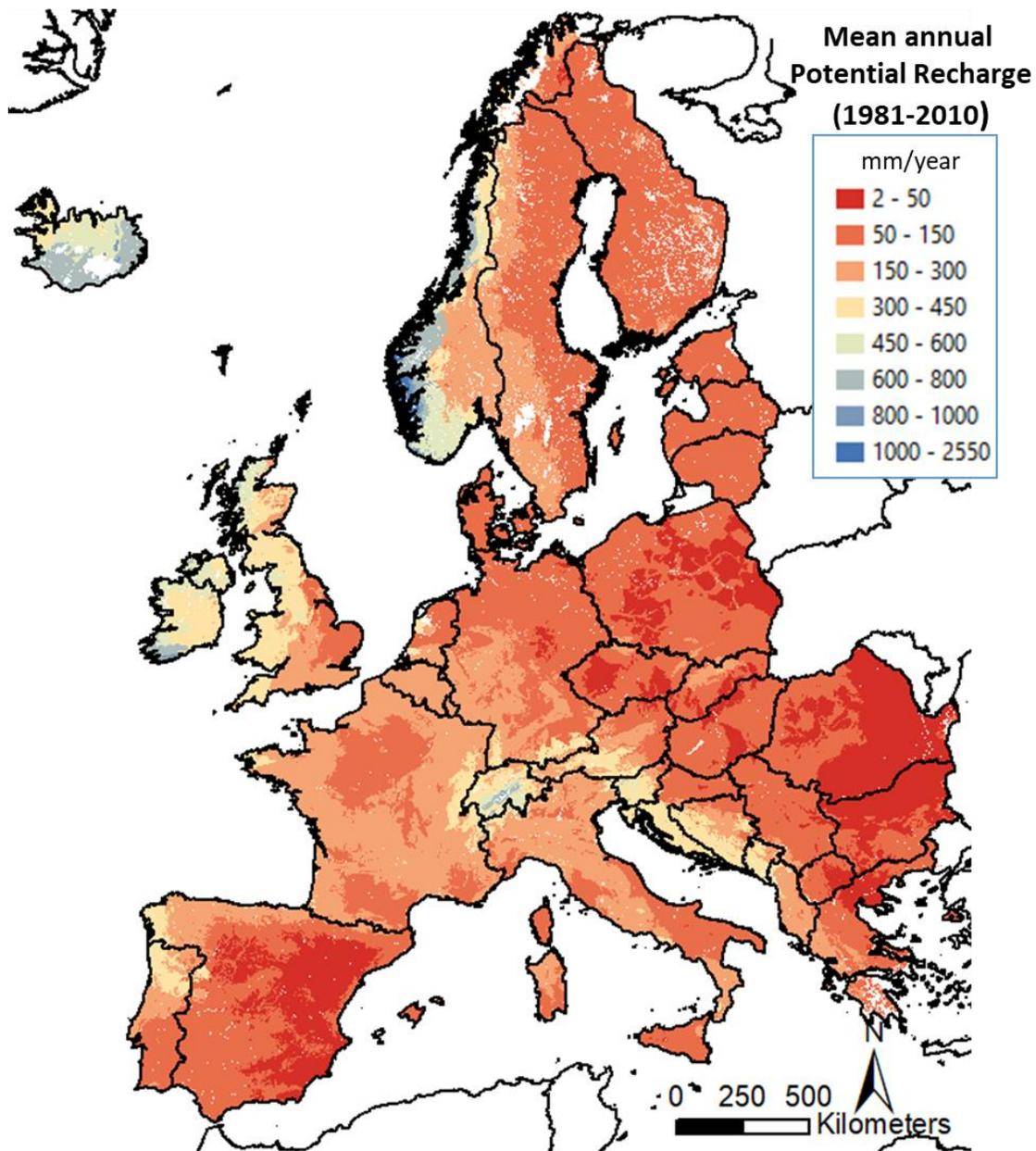
Figure 25: European Potential groundwater recharge map (1981-2010, hydrogeological unit scale)
