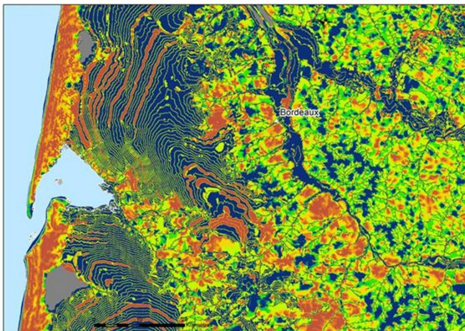
Figure 10: Terrace" effects produced by the slope calculation
